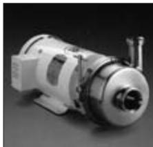
*Thomsen* is the name to turn to when you need a quality economical stainless steel sanitary centrifugal pump. There are four models to choose from with flows up to 500 gpm. The clamp head design permits 360 degree outlet rotation. An investment cast four blade impeller delivers a smooth steady flow. Internal, external and special seal combinations are available.
